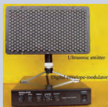
An audio spotlight prototype by the Kakamura Laboratory at the University of Electro-Communications, Japan
