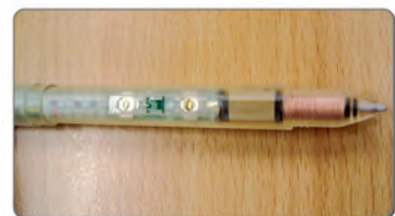
■ A transparent stylus with the pressure spring, coil and switches in view
